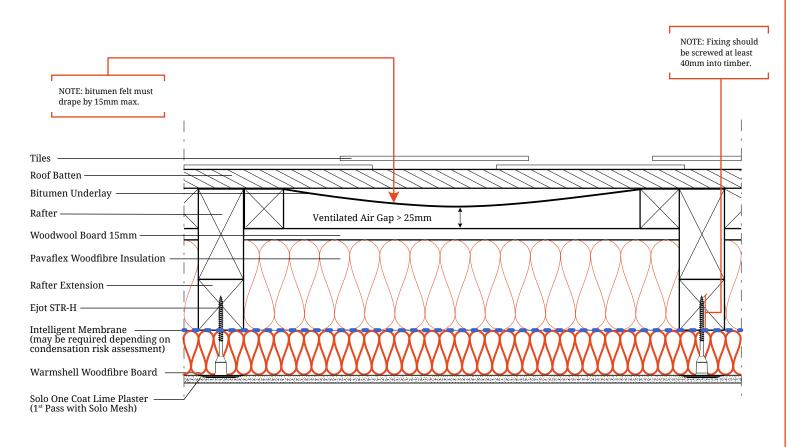
Retrofit Pitched Roof with Existing Bitumen Underlay
