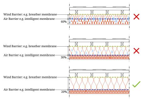
Retrofitting insulation to an existing roof where the tiles are not being re-laid requires careful inspection. Bitumen felt and some other types of underlay may not be breathable, in which case the ventilation strategy must be altered to allow ventilation underneath the felt (see detail ROOF 001), rather than across the top, as is more common.
