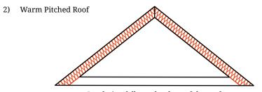
*Insulation follows the slope of the roof.*
