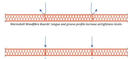
Woodfibre insulation boards without a tongue and groove have increased levels of thermal bypass.
