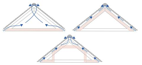
As a general rule, the material with the highest vapour resistance must be on or near the warm side, and the material with the lowest vapour resistance should be on the cold side. Membranes are popular as they make following this principle simple, but it can also be achieved without using membranes. Where membranes are used, they must be installed without gaps or tears, and should be bonded at the edges to the walls.
