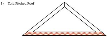
Insulation follows the line of the horizontal ceiling.
