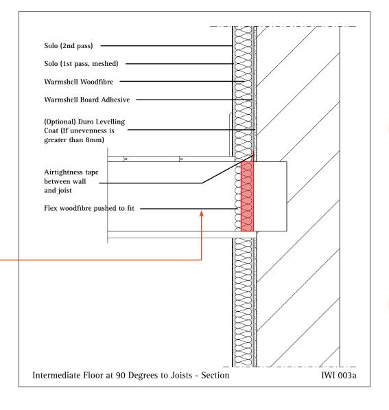
It is very important to achieve good levels of airtightness around the joists, either with airtightness tapes, or with Solo plaster, before installing the insulation.
