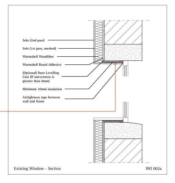
It is important to remember by fitting internal insulation there is less heat getting into the wall. This makes the wall, including any exposed uninsulated surface, colder than before and more likely to result in the formation of condensation on the exposed surface. Drawing Title
